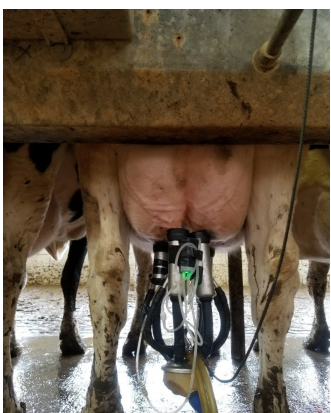
VaDia device attached to a milking claw to monitor milk flow
